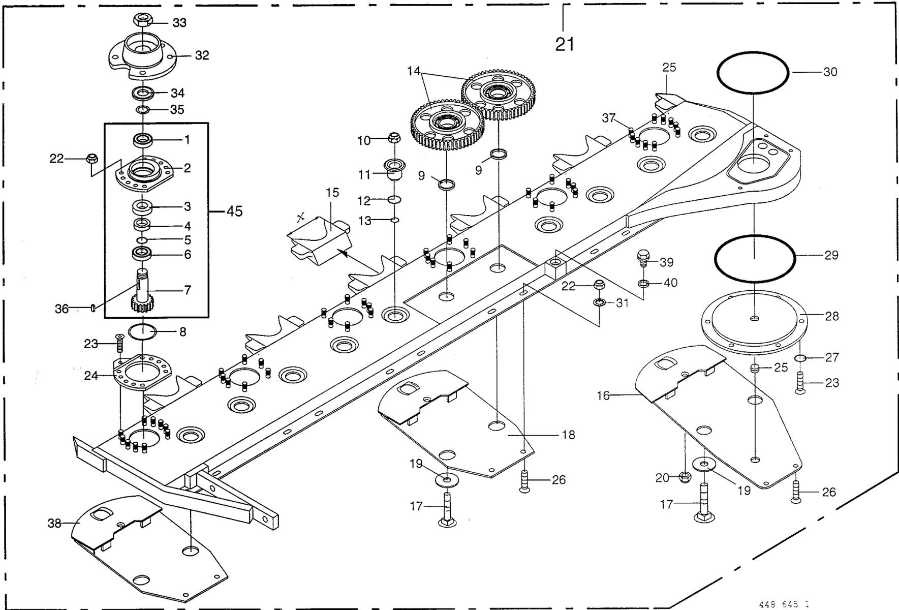
**Mower Beam with Bearings R/H - AMT 5000**
