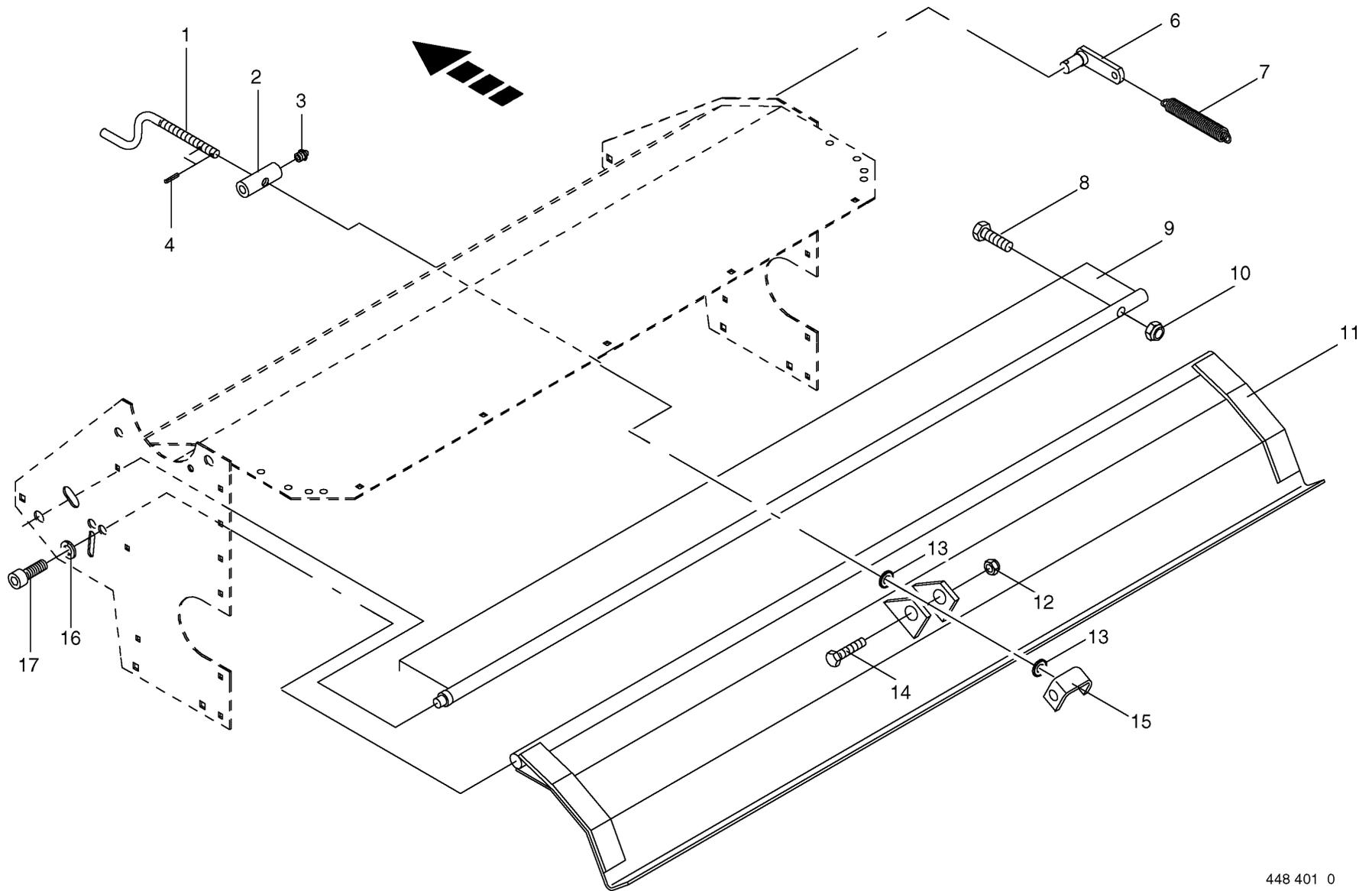
**Tine Conditioner Baffle Plate L/H - AMT 5000**
