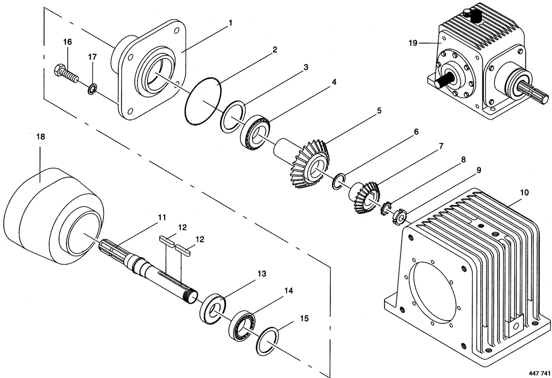
**Main Gearbox - Input Drive Shaft**
