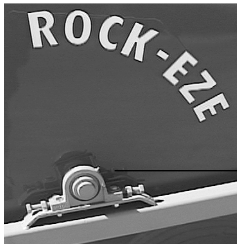
Figure 6.3 Rock wheel bearing lubrication zerk 1 of 2
