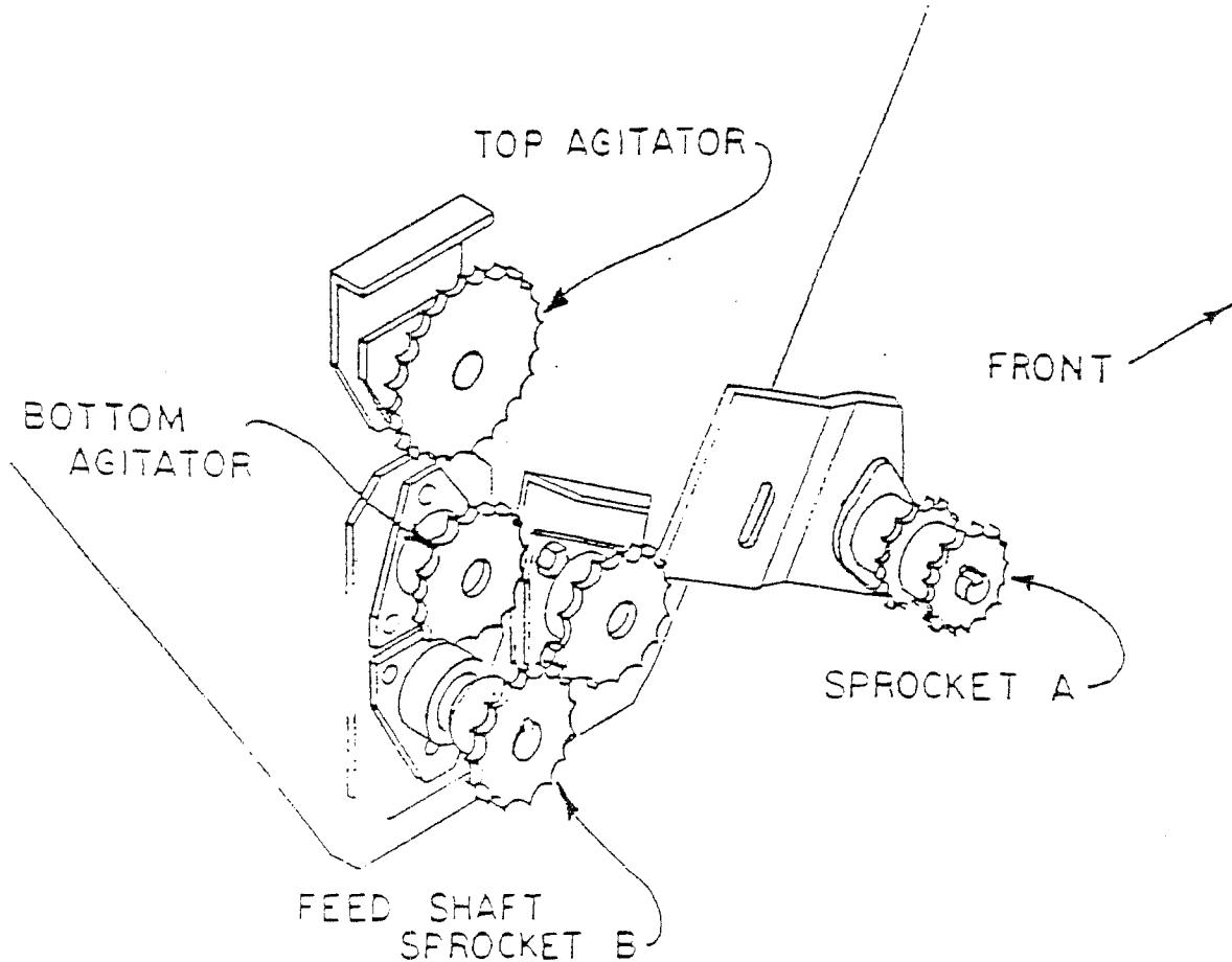
To obtain the desired seeding rate of the chaffy native grasses it may be necessary to adjust the feed shaft speed. The charts on pages 17 and 18 list the possible sprocket combinations and relative speed in revolutions per acre. Use these charts as a guideline in choosing the correct sprocket combinations. On a standard drill box, Sprocket A has 14 teeth and Sprocket B has 18 teeth. There are a 12 tooth and 24 tooth sprocket included in the shipping kit for the native grass attachment.
