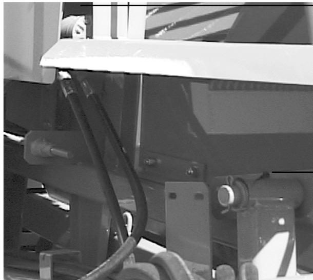
kicker rotor zerks (2), 2nd zerk is located near rear bearing
