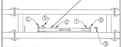
TRANSPORT LOCK ARMS CANNOT BE USED TO LOCK ONE RAKING WING. R.H. OR L.H IN ORDER TO WORK ON ONE SIDE ONLY BECAUSE THIS IS NOT ALLOWED.
