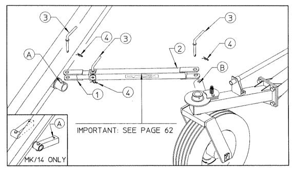
This is the assembly diagram for the MK16 and MK14. The row of holes on the arms is for when the rear axle is widened. Under no circumstances should the cylinders be operated while the transport arms are attached. The machine is now to be transported to the work site.
