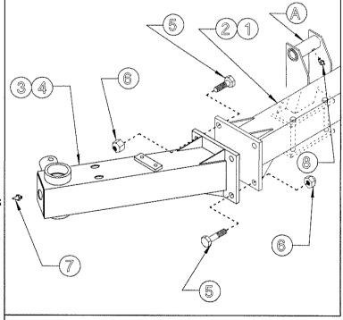
Item 8: 16/14 grease nipples  $M6x45^{\circ}$   $(1/4"x45^{\circ})$
