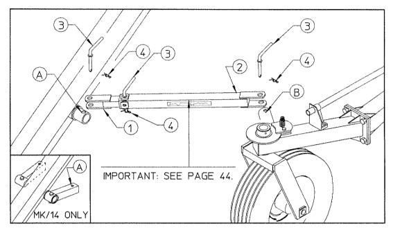
This is the assembly diagram for the MK16 and MK14. The row of holes on the arms is for when the rear axle is widened. Under no circumstances should the cylinders be operated while the transport arms are attached. The machine is now to be transported to the work site.
