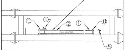
TRANSPORT LOCK ARMS CANNOT BE USED TO LOCK ONE RAKING WING. R.H. OR L.H IN ORDER TO WORK ON ONE SIDE ONLY BECAUSE THIS IS NOT ALLOWED.
